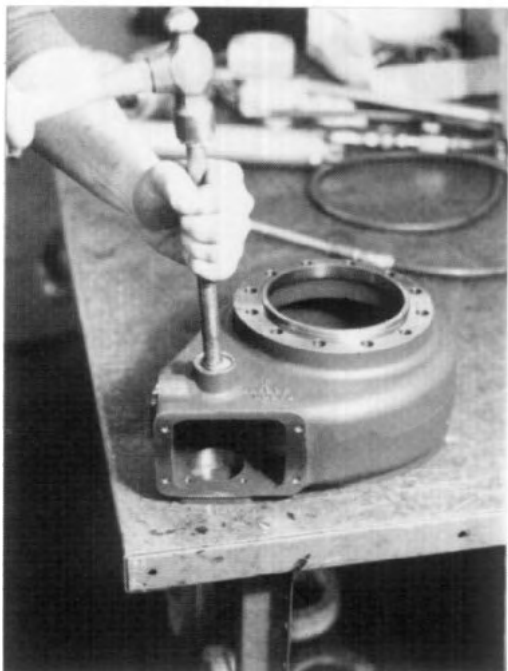
FIG. 6.2-6 If fitted with a PTO, drive the welch plug into the declutch housing, first coating with Permatex sealer. Be sure to use the correct housing, not mistaking the housing from the front drive declutch.
