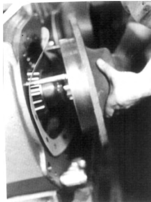
FIG. 6.4-15 Place carrier and gasket on locator studs and assemble into large opening in rear of housing.
