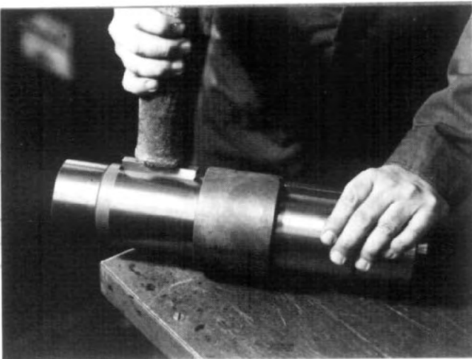
FIG. 6.1-2 While gears are warming, assemble keys into keyways in intermediate shaft. These should be a light drive fit and a soft brass drift may be used.
