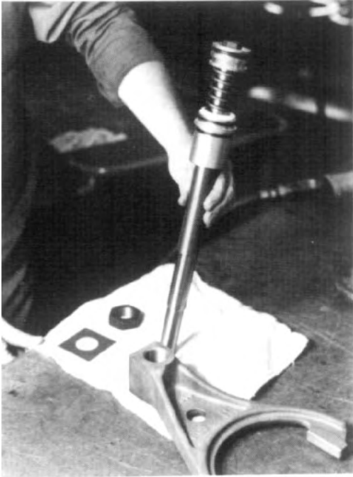
FIG. 6.6-1 Assemble shift shaft with small O-ring, adapter tube with O-rings, spring, stop ring, piston with O-ring, lockwasher and locknut together as shown.
