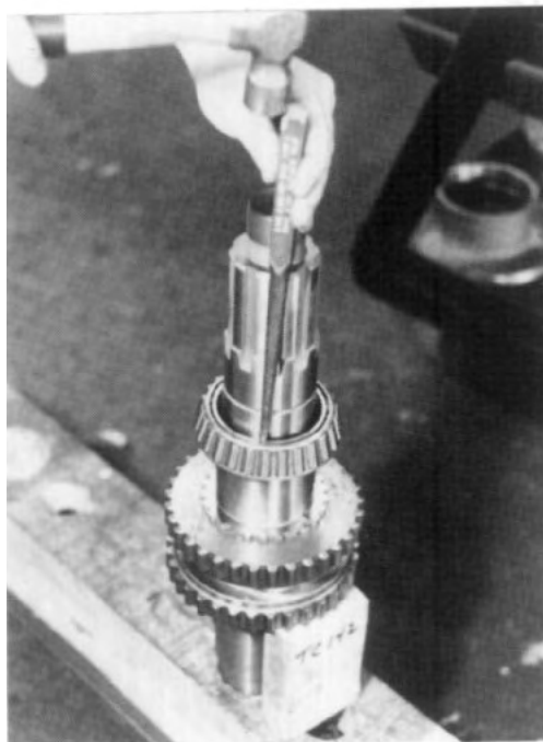
FIG. 6.3-3 Tap smaller gear internal bearing cone lightly to get started on shaft, when aligned it should slip relatively easily.
