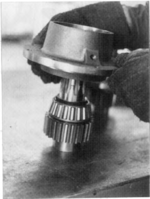
FIG. 6.7-2 Place output shaft bearing cones in heater for approximately 3 minutes. While waiting assemble snap ring and clutch gear to output shaft. Wearing heat resistant gloves assemble bearing cone to output shaft, add spacer ring between cones and lower carrier with cups onto shaft. Add second bearing cone to shaft, turn carrier to be sure it is free.
