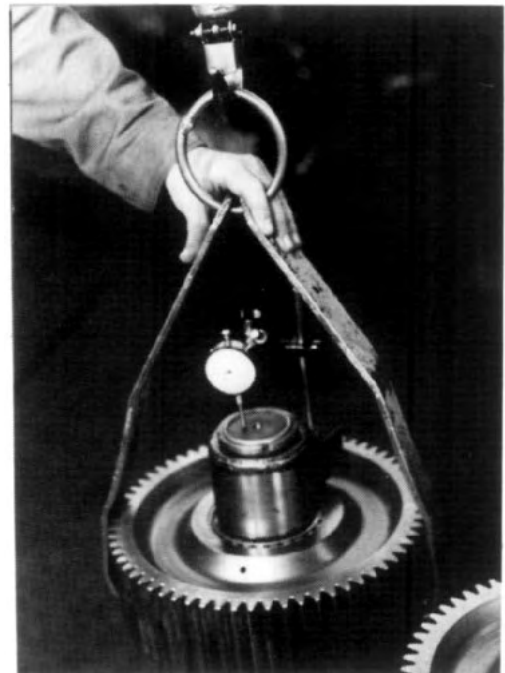
FIG. 6.3-11 Assemble tool number 866 650 to shaft and gear and check end float in bearings with dial indicator as shown. Total end float should be between .003 and .008 inches. Replace spacer between gear bearings if necessary to provide correct end float.
