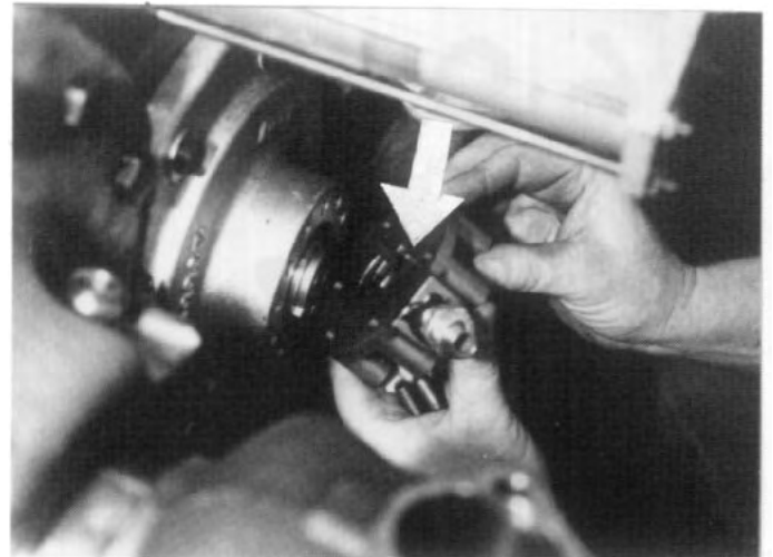
FIG. 6.8-4 Assemble pump end cap with 2 cap screws, just started, to carrier. NOTE - Be sure pin (arrow) on flat mating face of cap engages shoulder slot on end of pump. Turn pump assembly if necessary to place cap in correct orientation for plumbing.
